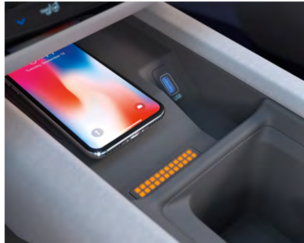
The wireless charger port features Parametric Pixels that signal the charge level of your smartphone at a glance.
